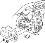
Fit the bar over the bar bolts. Place the bar in its rearmost
